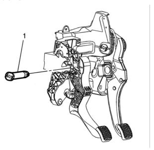
Apply GM Super Lube Part Number 12346241 (in Canada use 10953474) or equivalent around all the gaps on the clutch pedal pin (1) in the illustration above.
