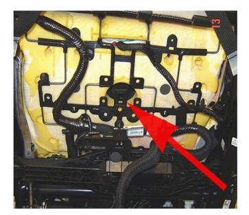
9. Inspect the tab on the bottom of the seat in the fan cavity area for evidence of contact with the fan blade.
