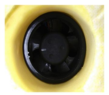
Reposition the fan to achieve the proper seating as shown. DO NOT PULL EXCESSIVELY ON THE FAN – IT MAY BECOME UNSEATED.
