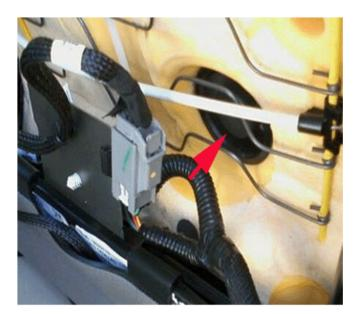
10. Inspect the under seat harness for excessive length and interference with the fan blade.
