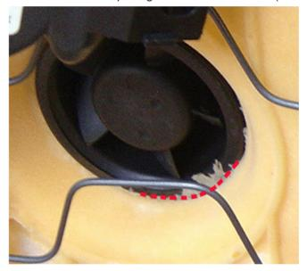
• If flashing is present, use a appropriate tool to trim the foam as shown.
