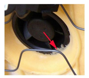
11. Inspect the foam seat cushion around the fan opening for excessive material (flashing).
