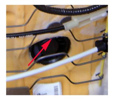
12. Inspect the felt attached to the foam seat cushion for excessive material that may contact the fan blades and trim as required.
