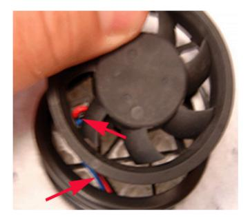
14.2. While returning the fan housing to its sheathing, rotate the motor to a position that minimizes the slack in the wires. Tuck the wires along the outside of the housing, eliminating the potential for them to interfere with the fan blades.
