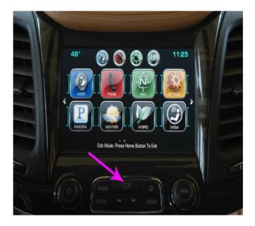
8-inch (203 mm) motorized color touch-screen display with concealed storage space behind the display and a USB port. Press and hold the button to open/close the door.
