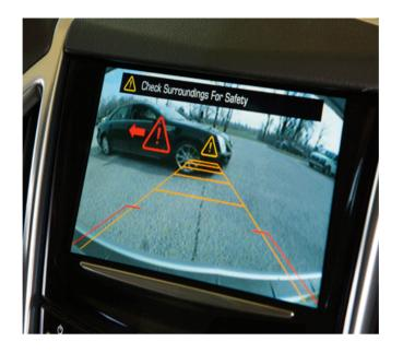
Displayed images may be farther or closer than they appear. The area displayed is limited and objects that are close to either corner of the bumper or under the bumper do not display. A warning triangle may display on the RVC screen to show where the Ultrasonic Rear Parking Assist (URPA) has detected an object. This triangle changes from amber to red and increases in size the closer the object.
