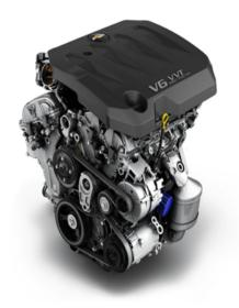
The 6-cylinder 3.6L flex-fuel with DOHC with VVT and DI — RPO LFX producing an estimated 303 hp (226 kW)
