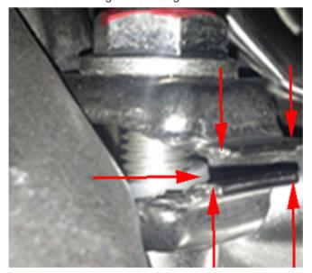
**Note:** The illustration above shows the ends of the V-band clamp with the gap.
