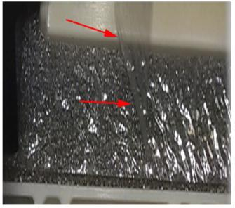
**Note:** Mylar strip peeling off the foam as shown in the illustration above.
