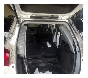
The cause of this condition may be that the dust/debris is working past the side door or liftgate sealing surfaces.
