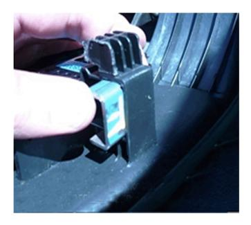
6. Install the two C shaped brackets from the Seat Side Cover Service Repair Kit into the mounting bosses of the new trim panel as shown above.
