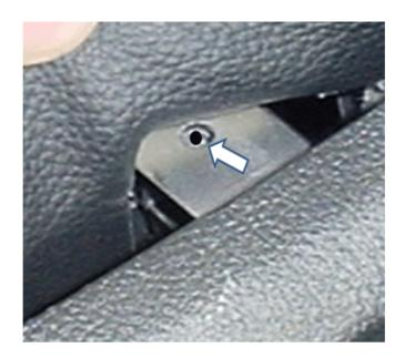
11. With the brackets aligned, mark the new screw hole locations through each hook bracket hole onto the plastic seat trim underneath.
