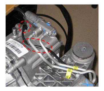
21. Reinstall the electrical connector to the limited slip differential valve and harness to the clip. Route the electrical harness under the pressure lines as shown.
