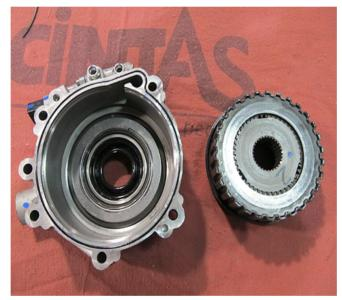
10. Remove the differential clutch pack from the clutch housing. Hold the housing in one hand and flip over to allow the clutch pack to fall into the other hand.
