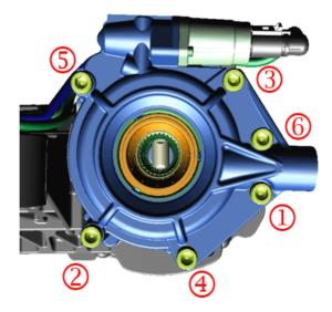
19. Reinstall the limited slip differential clutch bolts (Qty: 6).
