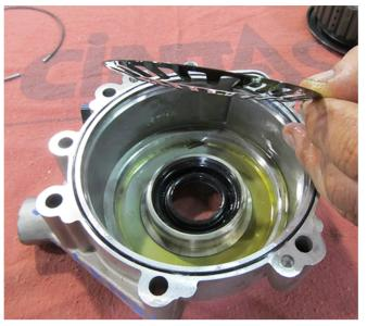
**Note:** If the piston spring is removed, ensure proper orientation when reinstalling. Spring fingers must be positioned as shown above.
