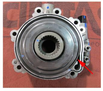
9. Remove the retaining ring that secures the differential clutch pack to the clutch housing.
