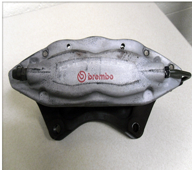
Finish Removed by Wheel Cleaner
