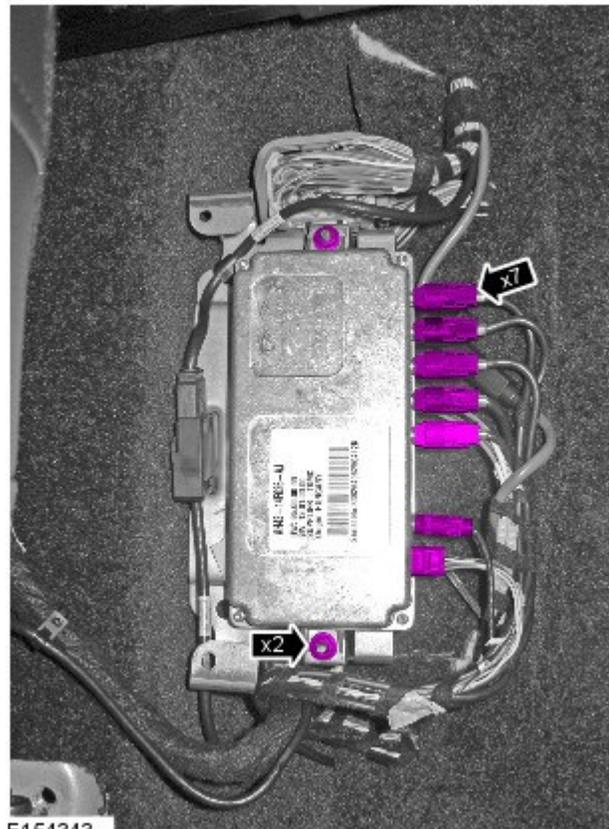
5. Install the new Camera Control Module.
