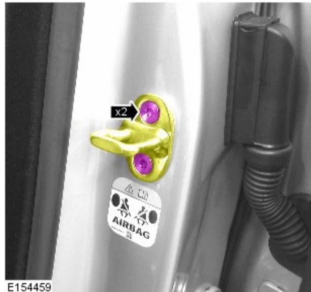
7. Adjust the door by the required amount to achieve the tolerances stated in step 2 above.
