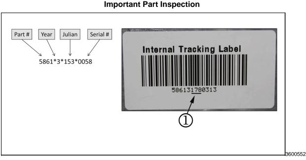
Generator Control Modules (GCM) with part number 24269448 or 24266403 require an inspection prior to installation in a vehicle. GCMs with part number 24267940 or 24267941 do NOT require inspection prior to installation in a vehicle.
