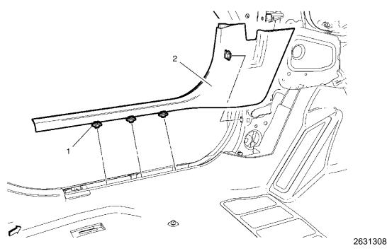
2. Open the driver side door and remove the front side door sill trim plate. Refer to *Front Side Door Sill Trim Plate Replacement* in SI.
