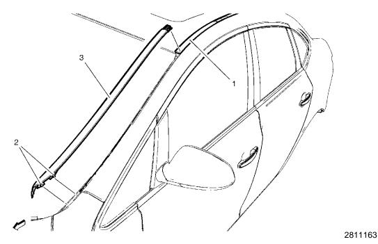
1. Using a body trim tool or equivalent, remove the windshield side reveal molding. Refer to *Windshield Side Reveal Molding Replacement* in SI.
