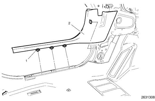
7. Install the front side door sill trim plate. Refer to *Front Side Door Sill Trim Plate Replacement* in SI.
