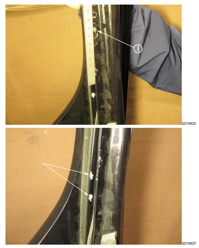
**Note**: The window reveal molding has a recessed flat area in the approximate location to mount the spacer.
