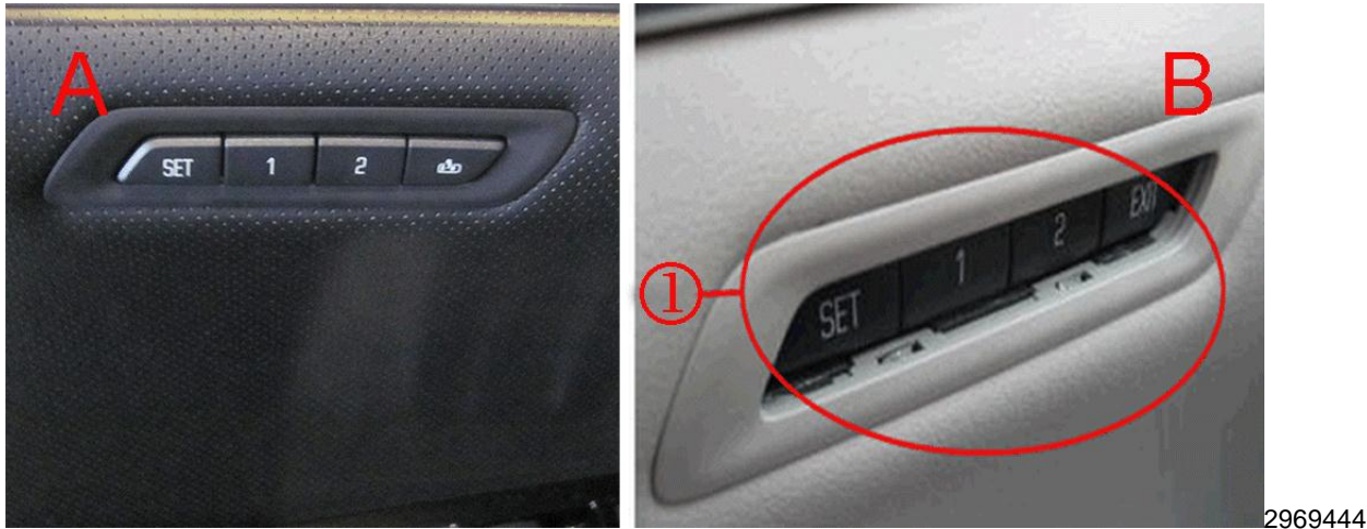
(A) Good driver seat memory seat switch. (B) Driver seat memory seat switch requires repair. The buttons (1) are pushed into the door trim panel.
