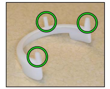
C The retaining ring is installed into the filler neck with the alignment pins <circles> facing toward the fuel tank.
