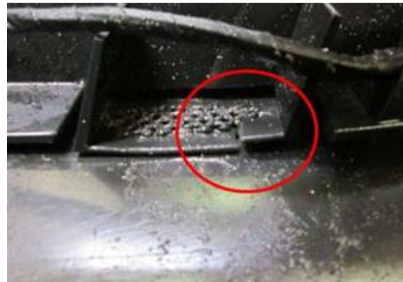
Figure 3. Broken mounting bracket
