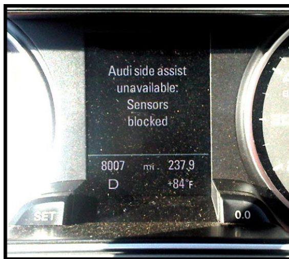
Figure 1. Audi Side Assist warning in DIS
