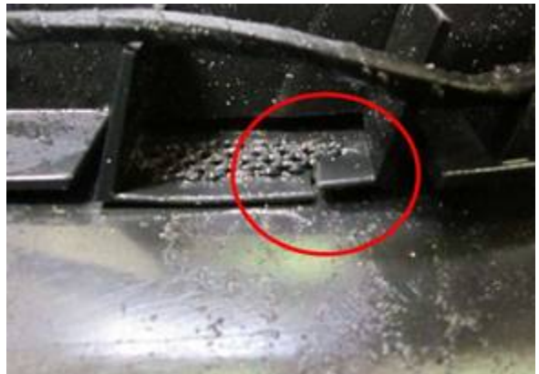
Figure 3. Mounting bracket broken
