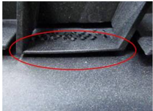
Figure 4. Mounting bracket loose
