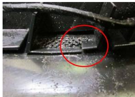
Figure 3. Mounting bracket broken
