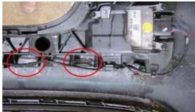
Figure 5. Bumper bracket weld locations with broken welds.
