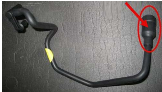
Figure 2. Updated ventilation hose with integrated filter.
