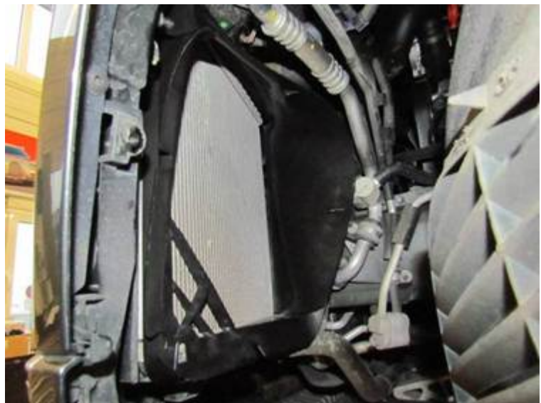
Figure 9. Exit air duct installed.
