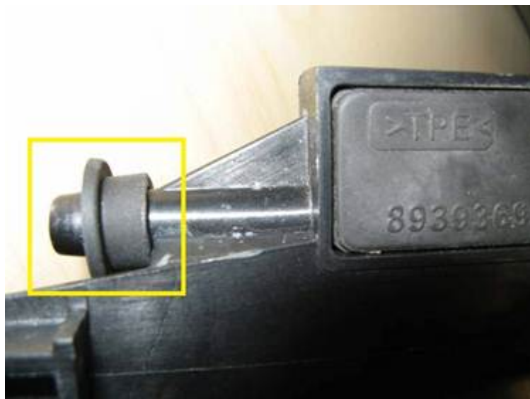
Figure 5. Ring seal installed on headlamp air tube.
