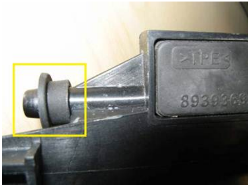
Figure 5. Ring seal installed on headlamp air tube.
