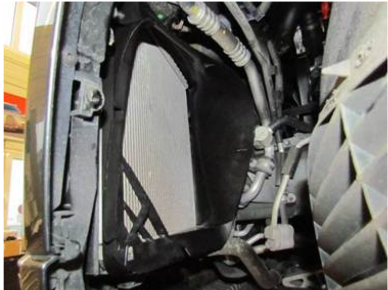
Figure 9. Charge air cooler exit air duct installed.
