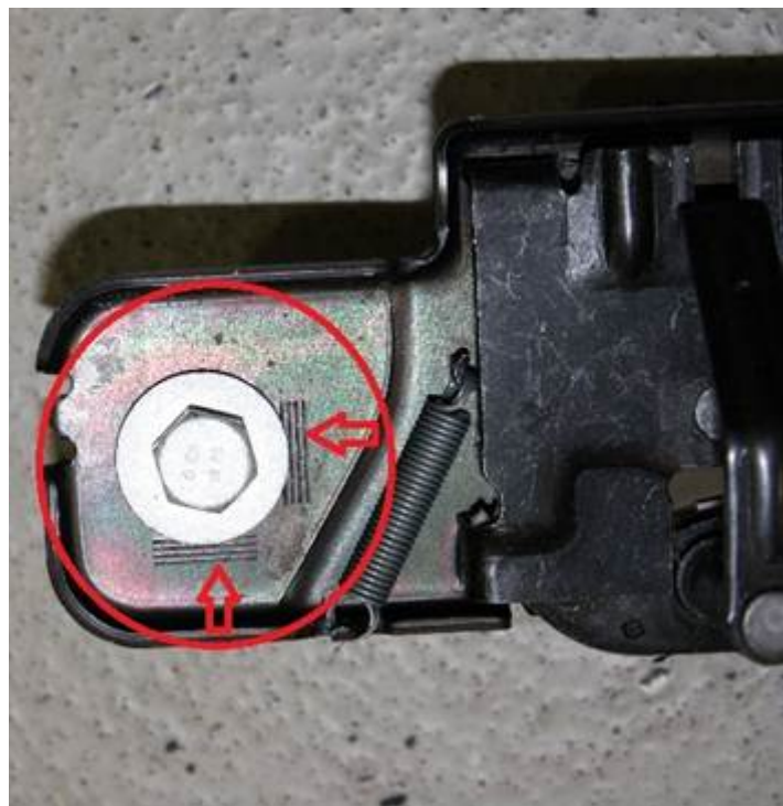
Figure 4. Power lid's motorized striker plate adjustability and serrated indicators.
