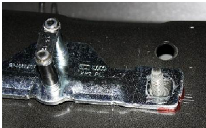
Figure 6. Manual lid style striker plate adjustability and serrated indicators.
