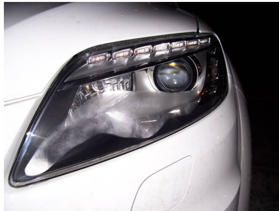
Figure 1. Moisture in headlamp.
