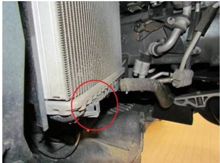
Figure 10. Lower exit air duct attachment point to charge air cooler.
