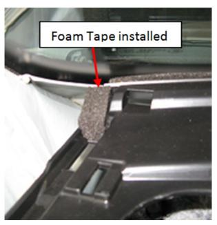
• Once the foam tape is in place, install the "A" pillar trim then install the speaker grille. Confirm the uneven gap has been eliminated. Another layer of foam tape or re-positioning of the first layer may be required to achieve the desired result.
