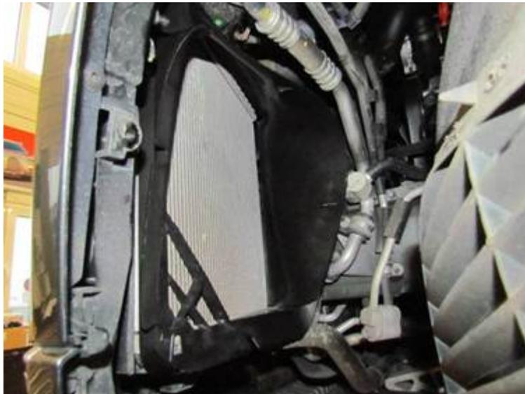
*Figure 11. Charge air cooler exit air duct installed.*
