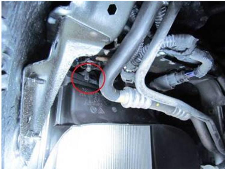
*Figure 12. View of exit air duct affixed to mounting hook.*
