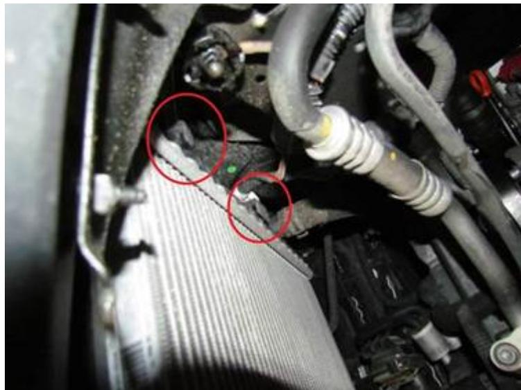
*Figure 10. Upper exit air duct attachment points to charge air cooler.*
