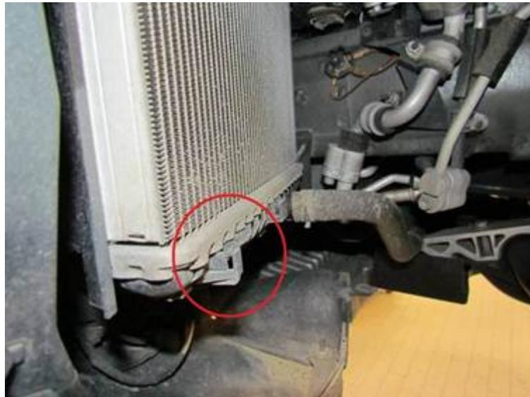
*Figure 9. Lower exit air duct attachment point to charge air cooler.*
