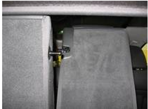
Figure 2. Armrest lock striker pin.
