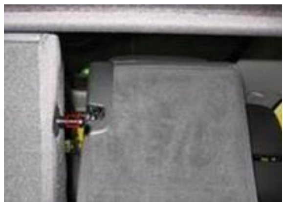
Figure 4. Area of striker pin to be lightly sanded.
