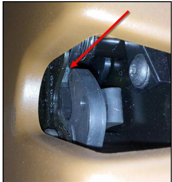
Figure 2. Arrow indicates direction to insert screwdriver. The latch is shown in the locked position.
