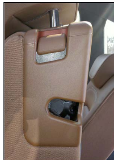
Figure 1. The rear center backrest latch and release lever.
