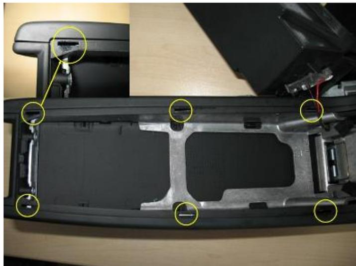
**Figure 2.** The mounting points into which the inner liner is slotted.
