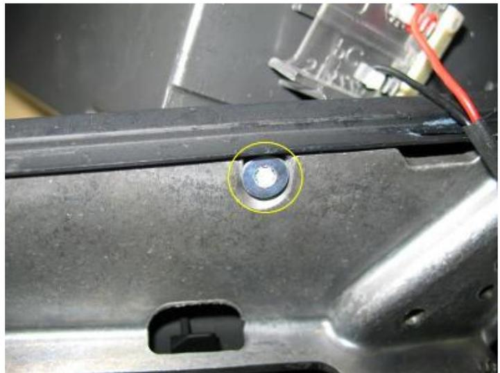
*Figure 4. A Torx bolt, which attaches the side trim.*
