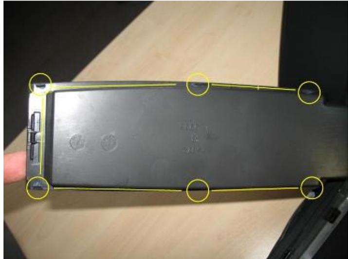
**Figure 1.** The inner liner of the center armrest, removed. Yellow circles highlight the areas to be lubricated.
