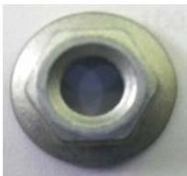
Original Nut, 12mm diameter flange surface
