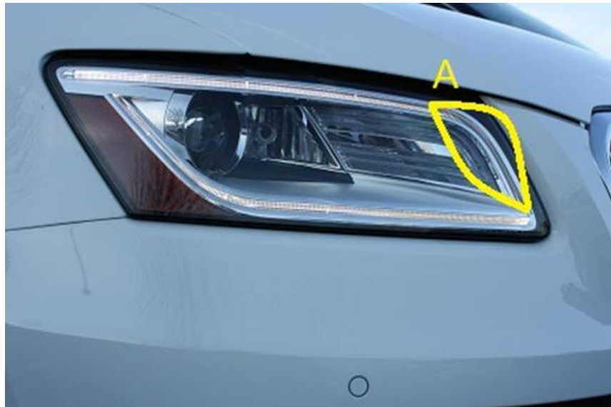
Figure 4. Upper light pipe perceived defect (A).
