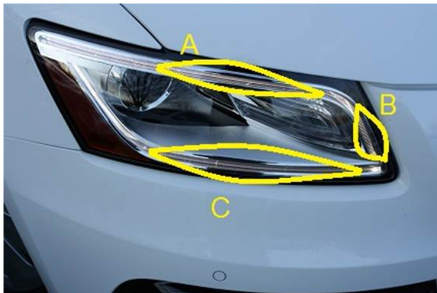
Figure 5. Upper light pipe perceived defect (A, B). Lower light pipe perceived defect (C).
