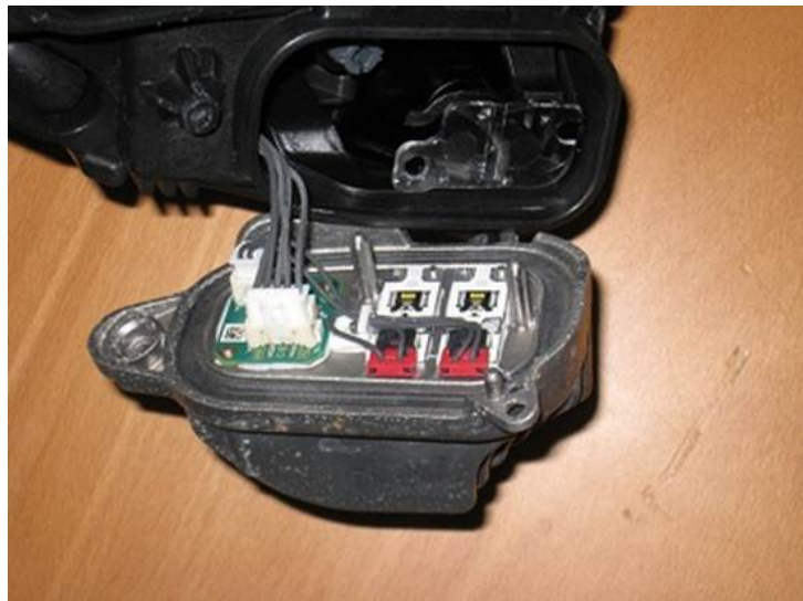
Figure 6: Dual surface mount LED unit exposed.
