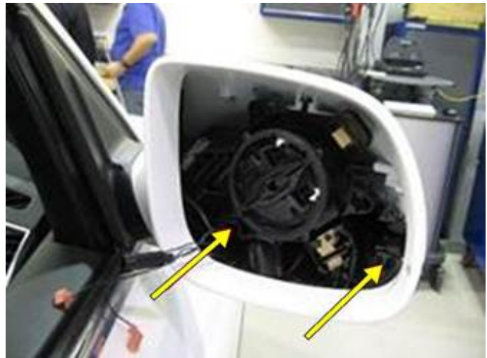
Figure 3. Location of the retaining clips.
