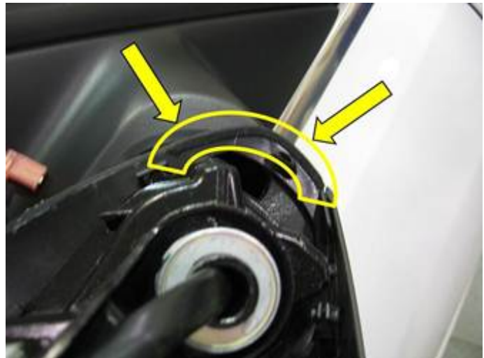
Figure 7. Felt tape applied.
