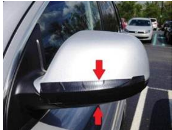
Figure 1. Application of tape over turn signal lamp.
