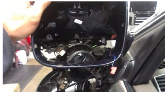
Figure 2. Removal of the mirror housing from the mirror base.
