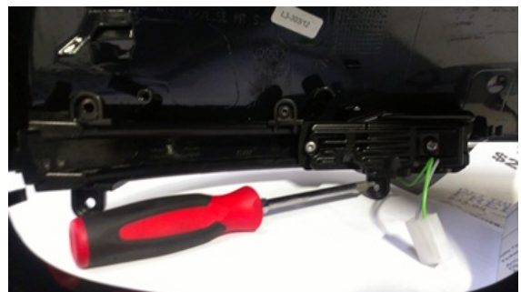
Figure 3. Removal of the turn signal lamp from the mirror housing.
