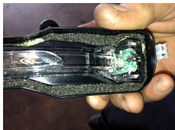
Figure 6. Turn signal lamp with sealing foam tape installed.
