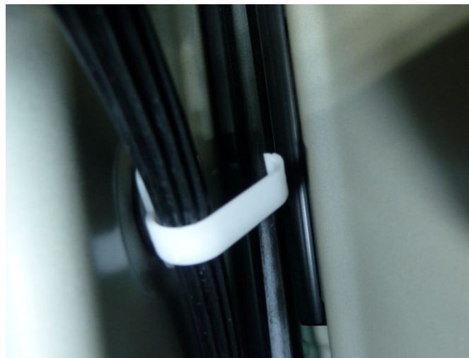
Figure 2. Clip as viewed from inside of the door panel.
