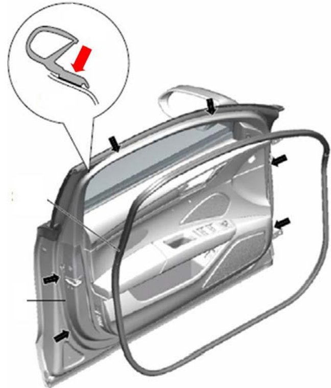
Figure 4. Apply force to the base of the seal (red arrow).
