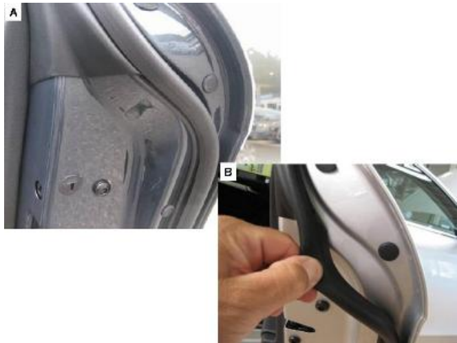
Figure 2. The door seal pressed to the door (A), and detached again (B).
