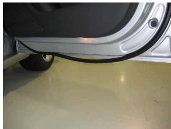
Figure 1. The outer door seal, partially detached.
