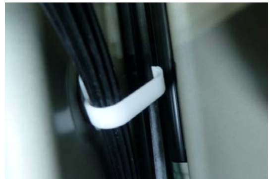
Figure 2. Clip as viewed from inside of the door panel.
