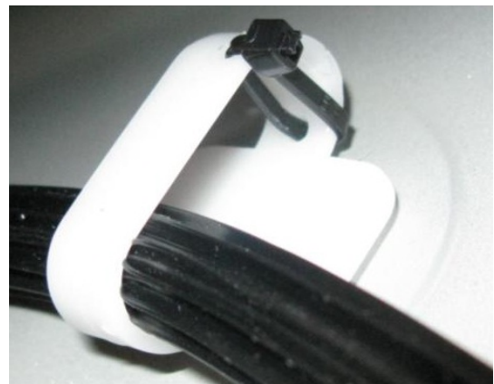
Figure 3. Clip with additional holes and zip tie.
