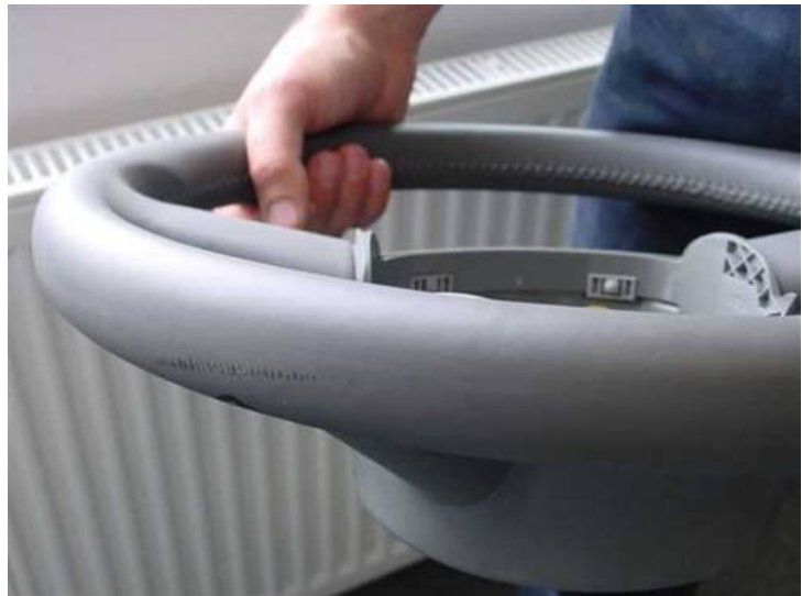
Figure 2. Example of damage from external impact.
