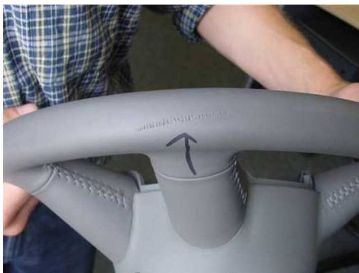
Figure 1. Example of damage from external impact.
