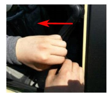
3. Pull the door weather strip to rework position.
