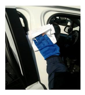
2. Wipe to remove adhesive residue using 3M Premium Sticker Cleaner – MS061 or equivalent if available. **Important:** Do not spray the adhesive remover on the body directly.
