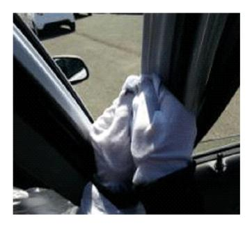
Important: Do not spray the adhesive remover on the body directly.
