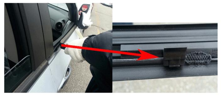
FOR T300 MODEL: Lower the door glass window fully and remove the door glass molding with special tool. (FRT LH/RH, RR LH/RH)
