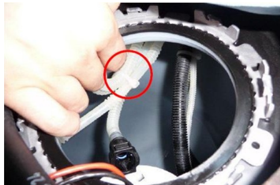
Figure 6. Curved fuel lines, fuels supply pipe, and fuel line tied together with tire wrap.
