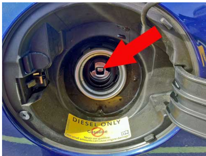
Figure 1. Misfueling guard, indicated by red arrow.
