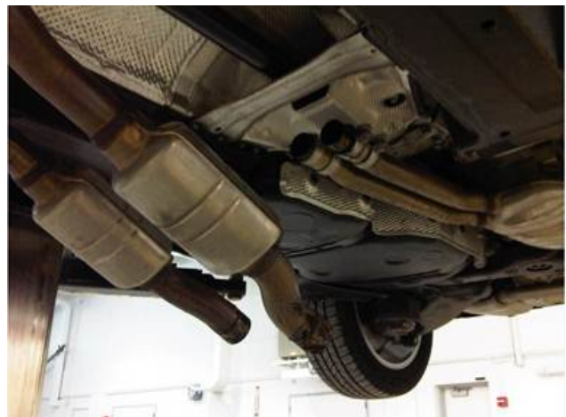
Figure 1. Lowered catalytic converter pipes
