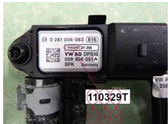
Figure 1. Date code on sensor in year, month, day format (example shows March 29, 2011).
