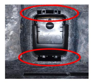
5. Add foam grommets onto each of the Christmas tree fasteners (if not present) prior to reinstalling back into the package shelf sheet metal holes. Use 1" X 1" block of Kent Adhesive Backed Shim Stock P/N P46510 or equivalent to create a foam washer(s) as needed. Fold the 1" x1" block over from corner to corner and carefully cut a hole in the center of the block to create a washer/spacer. See pictures below.
