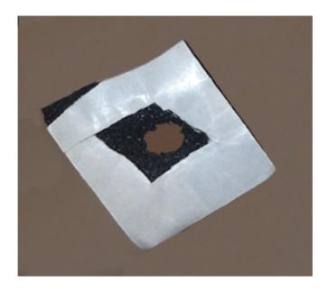
6. Add two ¾" by 1 1/2 " long by 7/16" thick of Kent Adhesive Backed Shim Stock (foam) P/N P46505 or equivalent centered between the retaining clips on the leading edge of the package shelf (behind/under the rear seat back). See picture below.
