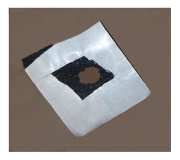
6. Add two <sup>3</sup>/<sub>4</sub>" by 1 <sup>1</sup>/<sub>2</sub>" long by 7/16" thick of Kent Adhesive Backed Shim Stock (foam) p/n P46505 or equivalent centered between the retaining clips on the leading edge of the package shelf (behind/under the rear seat back) see picture below.
