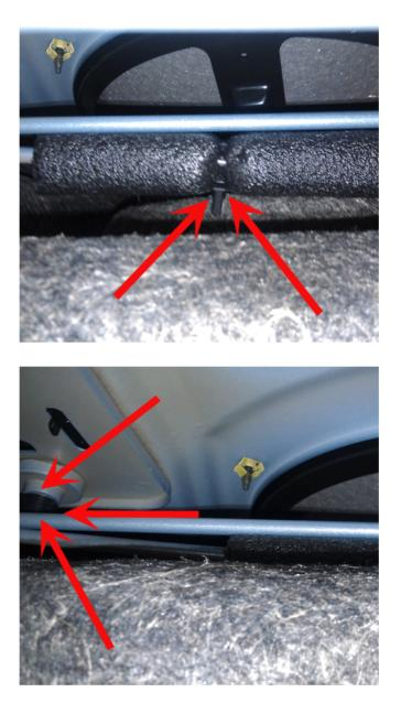
4. Add felt onto the package shelf trim opening to prevent movement between the trim and the child seat tether cover if the felt is not present. Use Kent Adhesive Backed Flocking Tape p/n KT13295 or equivalent see pictures below.
