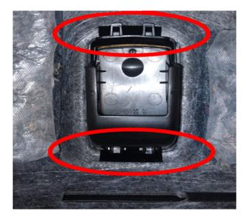
5. Add foam grommets onto each of the Christmas tree fasteners (if not present) prior to reinstalling back into the package shelf sheet metal holes. Use 1" X 1" block of Kent Adhesive Backed Shim Stock p/n P46510 or equivalent to create a foam washer(s) as needed. Fold the 1" x1" block over from corner to corner and carefully cut a hole in the center of the block to create a washer/spacer, see pictures below.
