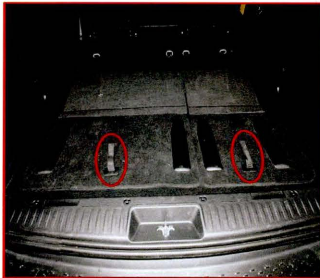
Fig. 1 Third Row Seat Bottom Pull Strap Locations
