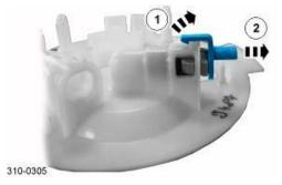
13. CAUTION: Make sure that the new O-ring seal is installed to the fuel tank fuel outlet mounting flange; failure to follow this instruction may result in damage to the vehicle.
