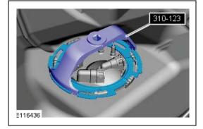
11.  $\triangle$  NOTE: Hold the fuel tank fuel outlet mounting flange above the fuel tank aperture and allow any fuel within the fuel tank fuel outlet mounting flange to drain back in to the tank before attempting to withdraw it through the vehicle interior.
