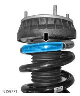
4. NOTE: When installing the new isolator sleeve, make sure the small end of the taper is closest to the end of the existing sleeve.
