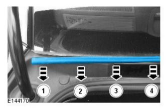
**4.** Using a suitable tool, remove the three (3) sections of adhesive tape from the rear window glass.
