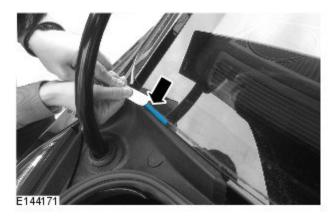
**5.** Using a suitable cleaning fluid, clean the lower edges of the rear window glass.
