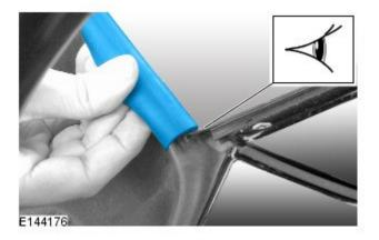
11. ONOTE: Make sure that the tape applies a suitable pressure on the rear window glass finisher until adhesion has been completed.
