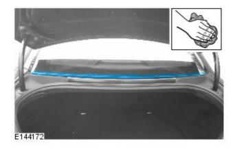
**6.** Using a suitable cleaning fluid, clean the outer faces and the channel of the rear window glass finisher.
