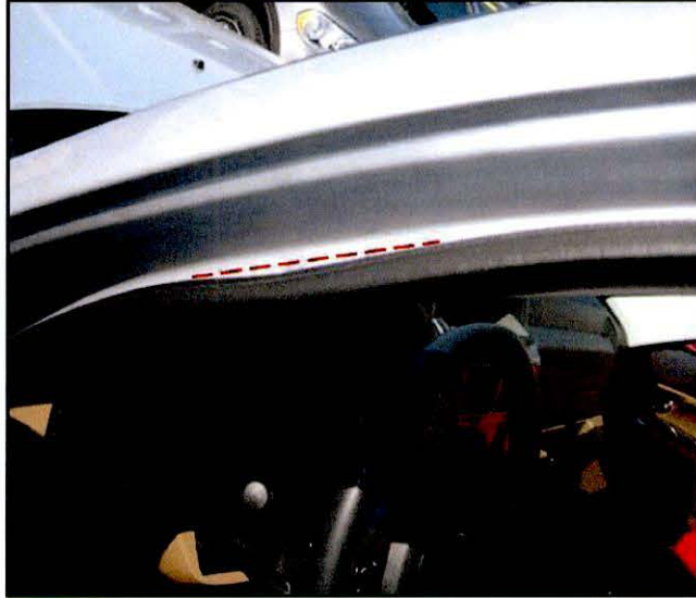
Fig. 1 Inspect Seal Placement
